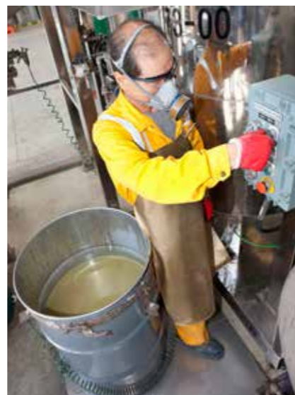
The Solvent Recovery System, Jotun Korea. Recycling solvents reduces costs related to the safe and sustainable disposal of chemical waste. This unit has the capacity to recycle 500 litres per day.
